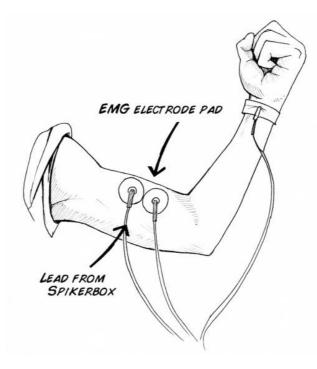
2. Hook up the EMG SpikerBox leads (the red and black alligator clips) to the two surface electrodes on your bicep.
