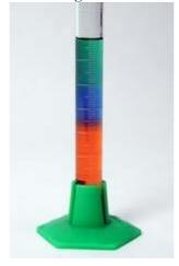
**Materials needed:** Liquids of different densities: honey, corn syrup, dish soap, water, vegetable oil, rubbing alcohol, graduated cylinder and Food coloring
